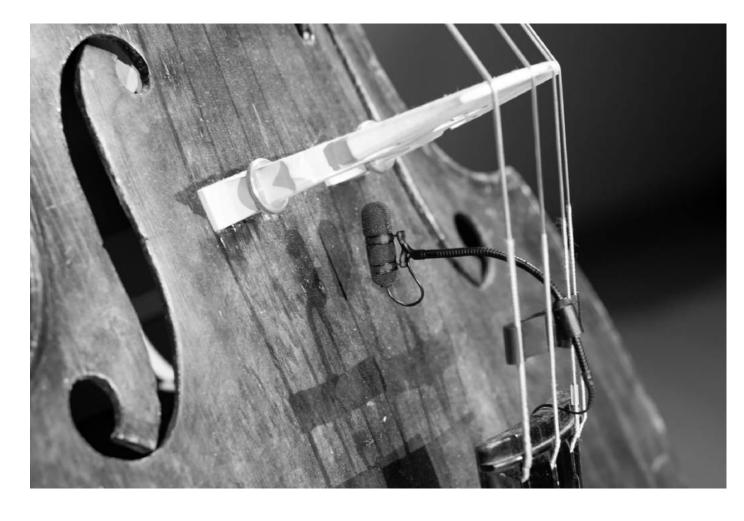
Preferably a radio transmitter should be used to send wirelessly the microphone signal to the mixer. If this option is not available, a long audio cable could be used but should stay out of sight.
